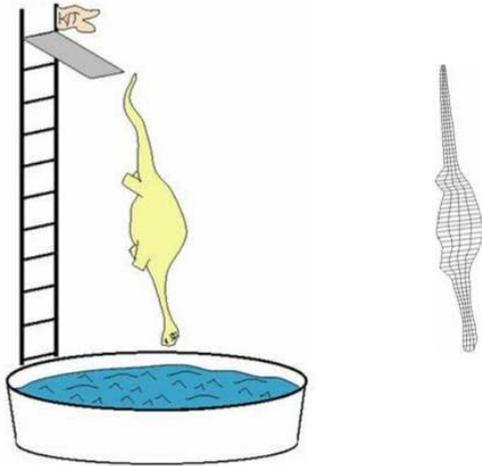
**Fig. 1:** Numerical modeling of any impact event begins with a discretization process. Projectile and target are divided into discrete blocks, or cells, each with associated individual sets of physical parameters. (Image courtesy of Gareth Collins).
