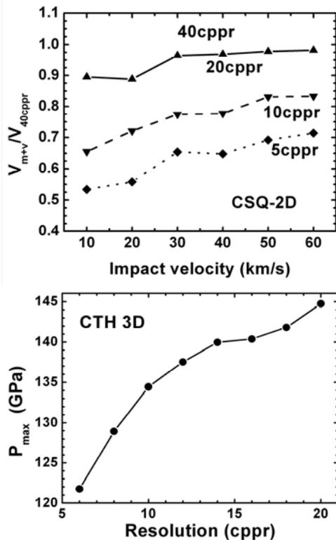
**Fig. 3:** *Upper:* Resolution effects in estimates of melt volumes for 2D simulations (using the hydrocode CSQ). From [6]. *Lower:* resolution effects in estimates of target's maximum shock pressures for 3D simulations (using the hydrocode CTH) [7].
