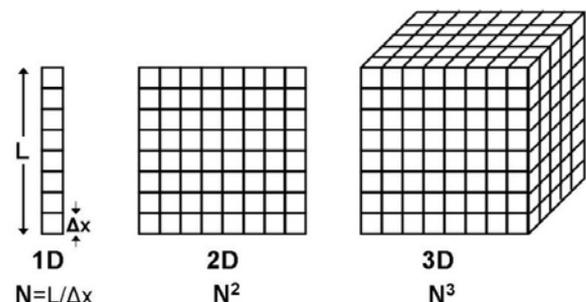
**Fig. 2:** Schematic of the number of cells involved in a numeric simulation for 1- 2- and 3-dimensions. L is the spatial scale of the simulation,  $\Delta x$  is the desired spatial resolution and N is the number of cell in any direction.
