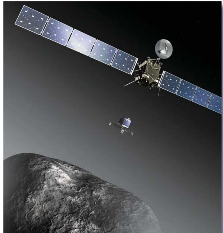
Artist's impression of the Rosetta orbiter at comet 67P/Churyumov-Gerasimenko. The Rosetta spacecraft measures 105 feet (32 meters) across including the solar arrays, while the comet nucleus is thought to be about 2.5 miles (4 kilometers) wide. The image is not to scale.
