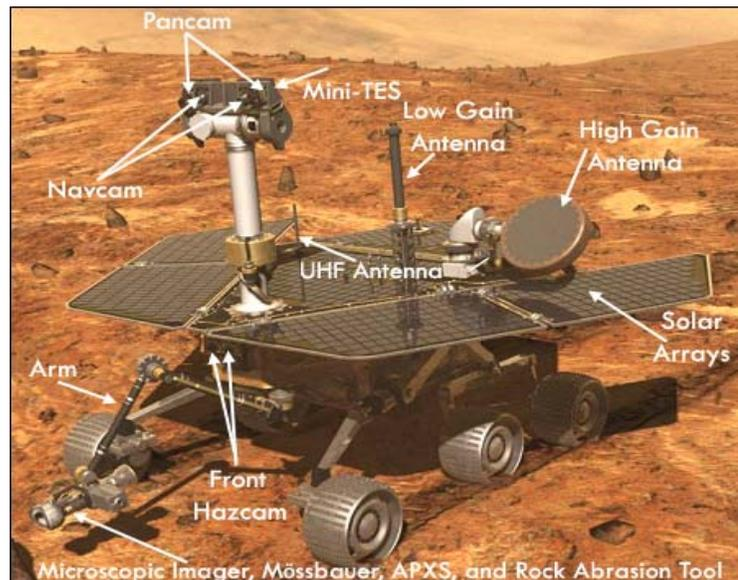
*Illustration of the Mars Exploration Rover and its science payload.*
